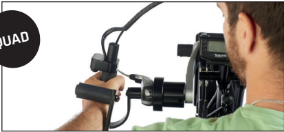
BATEC SHIFT LEVER. Shimano REVO 8 gear shifter.
