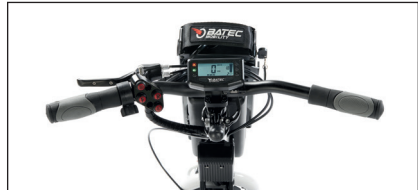
Monolever brake and accelerator handlebar for hemiplegics.
