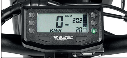
All-in-one LCD screen with speed selector.
