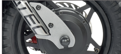
Removable right dropout to change inner tube and/or tyre easily.
