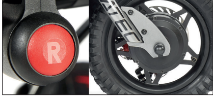
Brushless motor, 350 W nominal, 600 W maximum. Top speed of 20 km/h.
