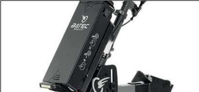
21,5 km* autonomy with 36 V – 280 Wh battery. 44 km* autonomy with 36 V – 576 Wh battery. 4A charger.
