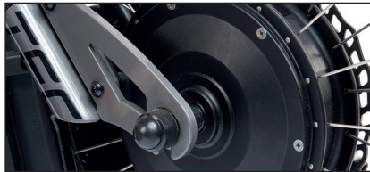
Removable right dropout for easy inner tube or tyre change.
