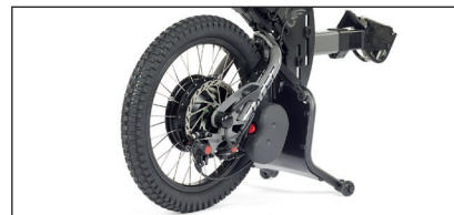
18" Wheel, ultra-grip tyre and aluminium double-wall rim.
