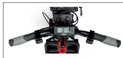
G&B handlebar option without levers for quadriplegics.
