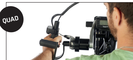
BATEC SHIFT LEVER. Shimano REVO 8 gear shifter.
