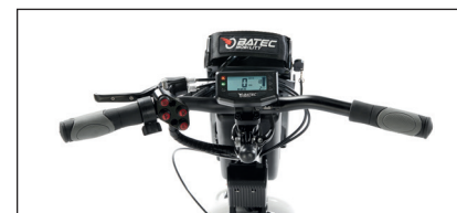
Monolever brake and accelerator handlebar for hemiplegics.
