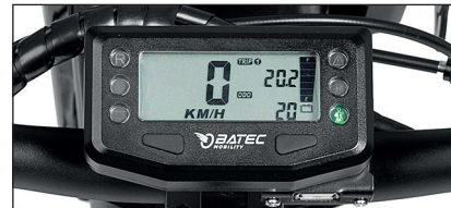
All-in-one LCD screen with speed selector.
