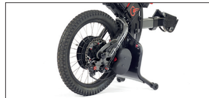
Ultra-grip tyre 18" x 2.40". Black double-wall aluminium rim.
