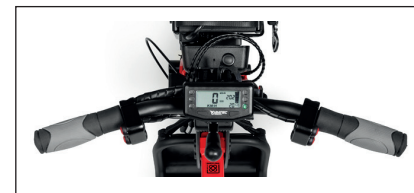
G&B handlebar option without levers for quadriplegics.
